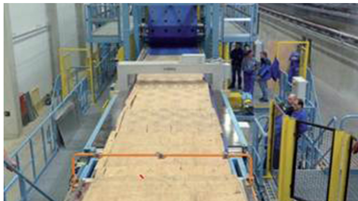
Permatek IM30 added to glue line during LVL manufacture.
